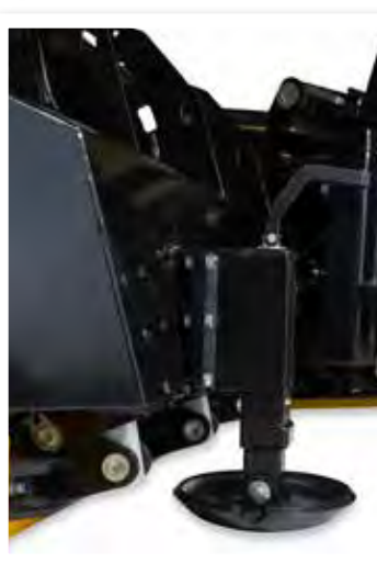
Skid shoes can be adjusted manually. The spring loaded cutting edge retracts if kerbs or similar objects are hit.
