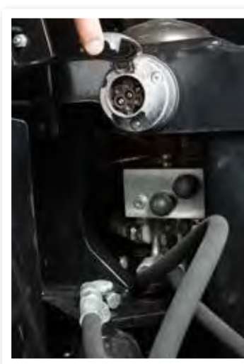
A quick coupling system makes it easy to attach and detach the electrics and control box from your tractor or wheel loader.
