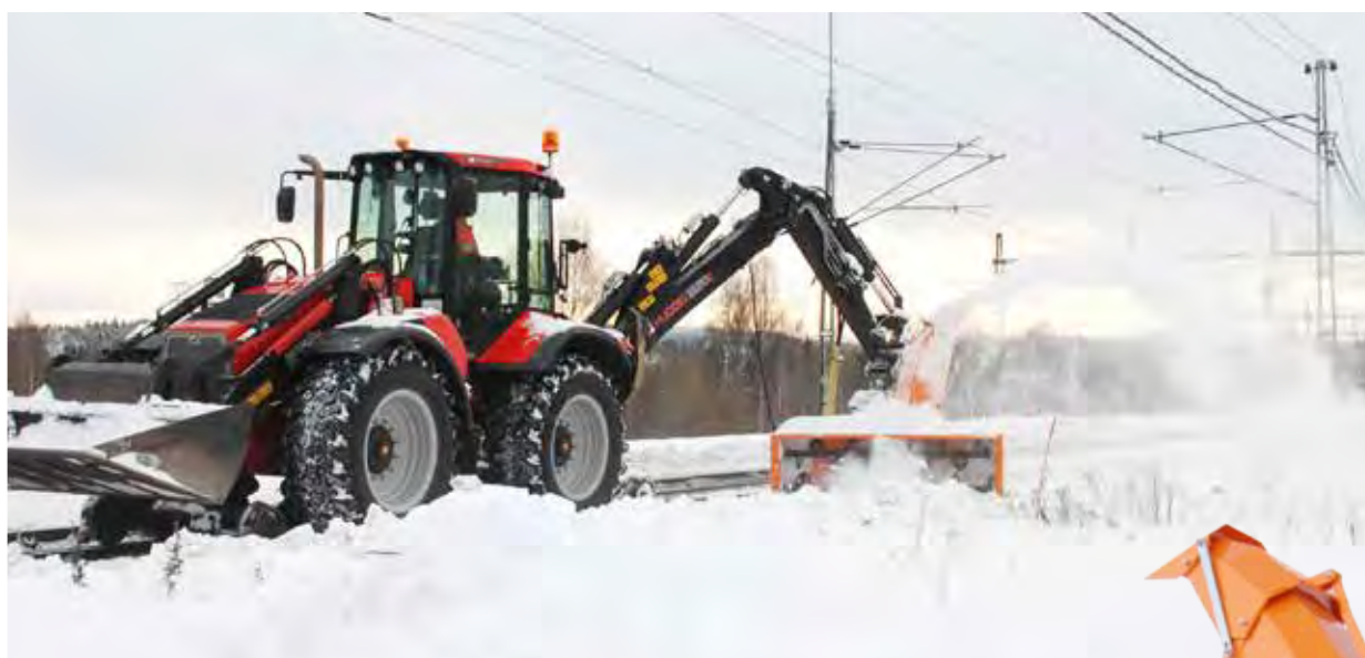
Trejon Optimal 2202H hydraulic snow blower seen here mounted on a Huddig 1260 for clearing snow from railway depots, stations and along the railway tracks.
