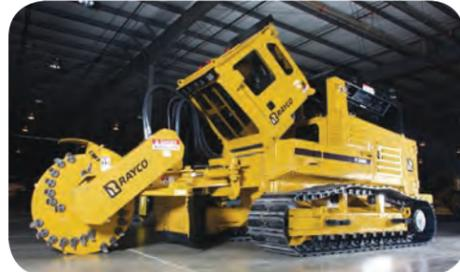
Tilt Cab for Access to Hydraulic Components
