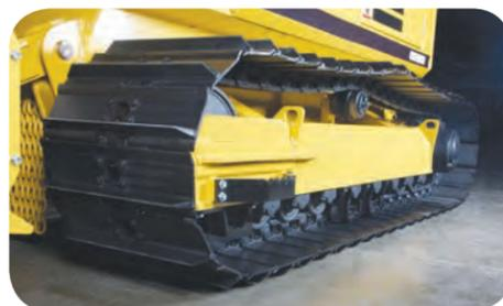
Heavy Duty Undercarriage with 2-Speed Final Drives
