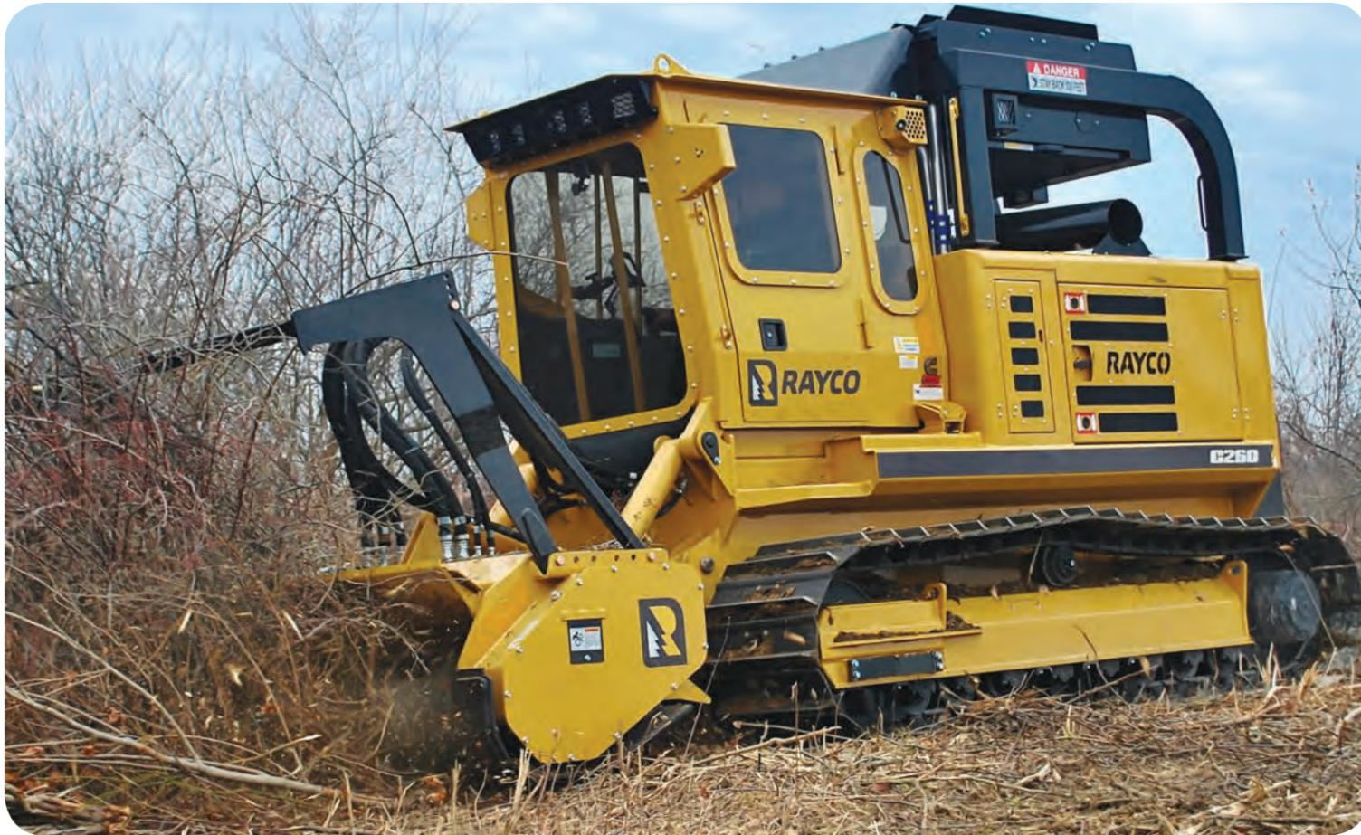
Rayco's C260 Crawler is a mid-sized mulcher that delivers 260 hp in a compact, low ground pressure package. A powerful Cummins QSB6.7L turbo diesel engine powers the C260. Rayco's exclusive elevated cooling design keeps engine and hydraulic temperatures within their limits in the harshest of environments. A reversing fan can be activated from the cab to clear the limbriser debris screens.
