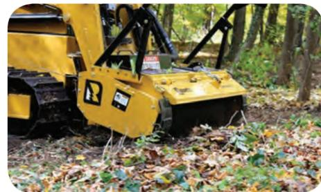
Predator Mulcher Head with Variable Displacement Motor
