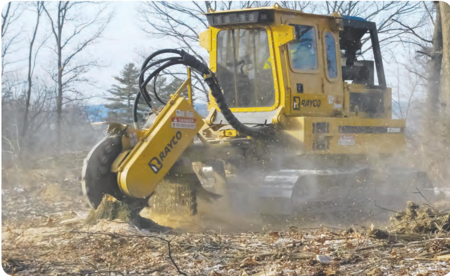
The T260 offers high volume stump removal in an easy to transport package. The T260 is a compact powerhouse for high production stump removal, with 260 hp in a chassis that weighs only 22,500 lb And an overall width of just 93-inch makes the T260 easy to transport without requiring permits. A 260 hp Cummins QSB6.7 turbo diesel powers the T260. It travels on a heavy duty steel track undercarriage with 2-speed final drives. The operator-
