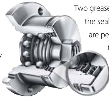
Two grease reservoirs located between the seals ensure that the seal lips are permanently lubricated and therefore prevent dry running. After extensive use the bearing housing itself can be changed quickly and easily with one bolt.
