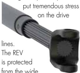
lines. The REV is protected from the wide angle drive shafts to the heat dissipating preset friction torque limiters. The multi-patented 80° ball and socket constant velocity joint distributes loads evenly, retains lubricant, reduces wear and keeps contaminants out. And for safety the patented articulated guard system maintains full coverage with the mating guard bell.
