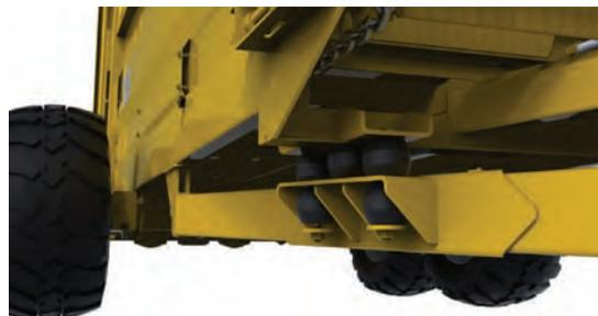
Tandem walking wheels cut uneven terrain in half with a massive unrestricted range of motion. All four wheels are always in contact with the ground surface. Coupled with a wide stance, these machines will ride over the roughest terrain with ease and control.
