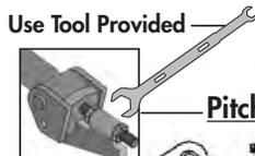
**NOTE:** For better performance, adjust pitch slightly down (lengthen rod length) to increase roller pressure.
