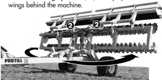
D. After fully opening the wings, extend the Transport Cylinders (#3) to completely lower the Pro-Till rear frame sections to the ground.
