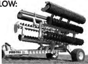
B. **Slightly** extend the Transport Cylinders (#3) just enough to remove the weight of wings off from the wing transport carriers. Do not lift more than needed.
