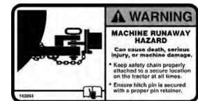
**WARNING:** *Negative Hitch Weight* may occur when raising or lowering the rear sections. If the unit is not properly attached to the tractor with a clevis hitch and safety chain, the negative hitch weight could result in the hitch pole to suddenly raise and the rear sections to come crashing down.
