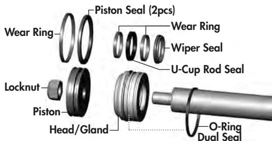
9. a) Inspect and replace all of the seals with new components.
