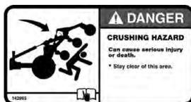
**WARNING/DANGER:** *Never disconnect Pro-Till from tractor if rear sections of machine are partially raised. Negative Hitch Weight may result, the hitch pole may suddenly raise and the rear section would come crashing down. Only disconnect when unit is on level ground in the proper transport or field position.*
