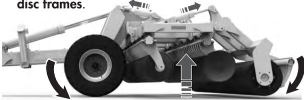
**NOTE:** It is important to fully raise the disc frames up as high as possible as it puts the rollers and wheels in the correct position for low transport.
