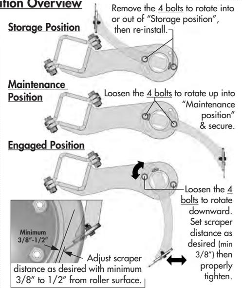
**Standard - Scraper Blade Kits** - c/w Bolts & Locknuts.
