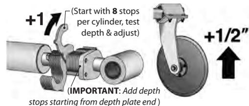
A typical recommended penetration depth of 2" is suggested. This depth, however, can be adjusted to the operators needs and preferences or based on different crop varieties and soil conditions.
