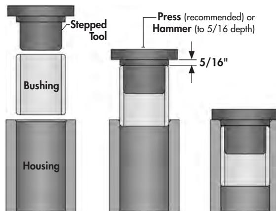
5. Ensuring the bushing is properly aligned, press into hole (preferred method) or hammer into position by striking the stepped tool.
