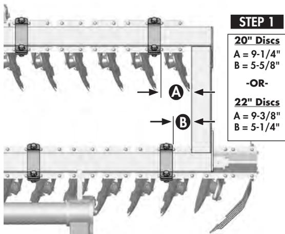
1. Gang section spacing starts by setting the distance from the inside RH Wing Frame to the edge of the first V-Clamp on front & rear gang sections. (Measurements - **A** & **B** in diagram).
