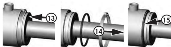
14. Loosen the clamp and remove.
