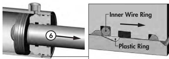
**Note:** Excessive force will not overcome a jammed ring and could damage the cylinder.
