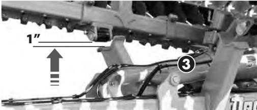
**⚠ IMPORTANT:** ***DO NOT** fully extend the transport cylinders at this point. Follow proper procedures to prevent possible equipment damage or failure.*
