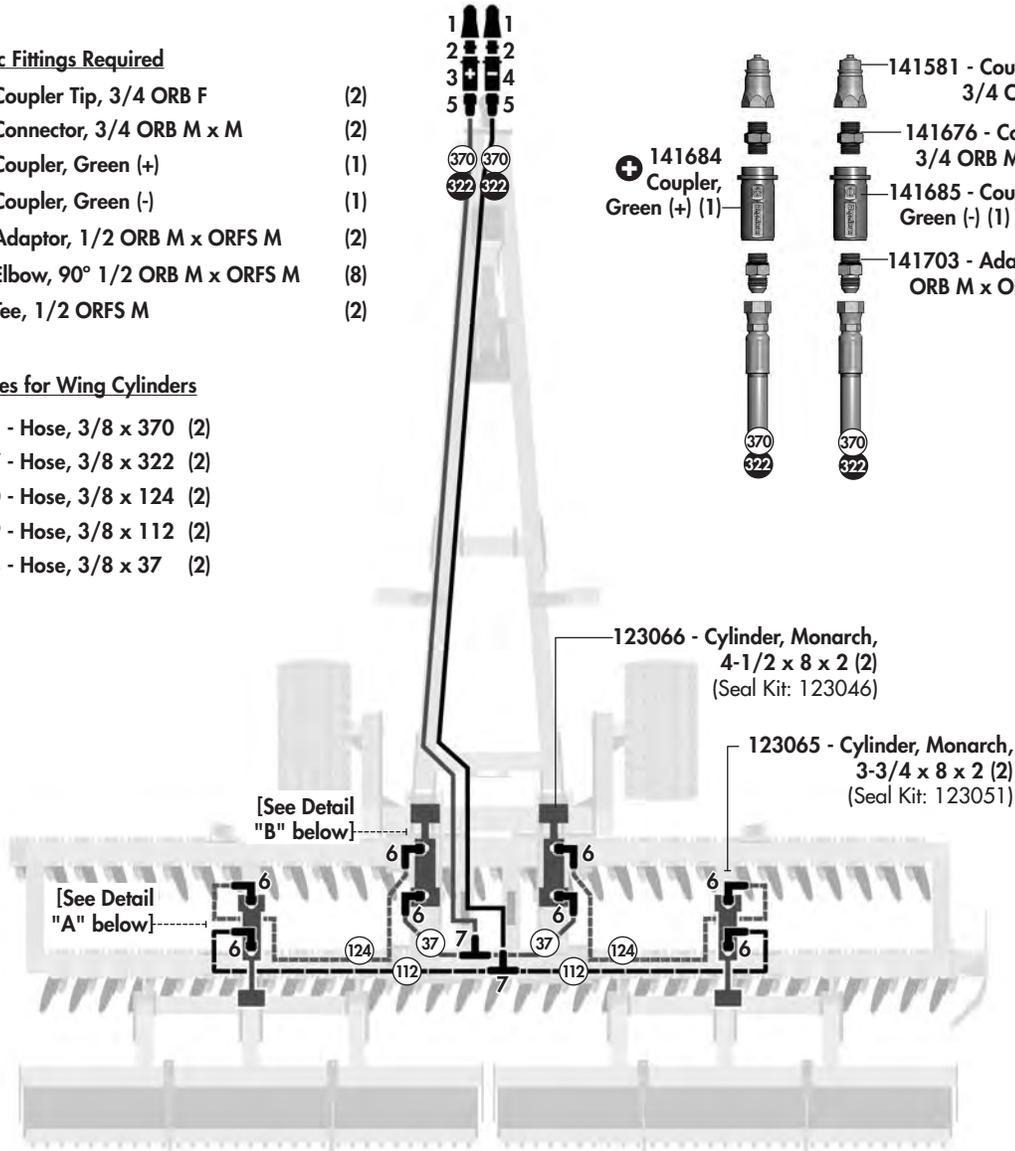
Detail A - LH Roller Cylinder Configuration (RH is Opposite)
