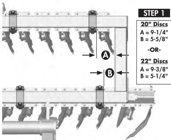
1. Gang section spacing starts by setting the distance from the inside RH Wing Frame to the edge of the first V-Clamp on front & rear gang sections.
