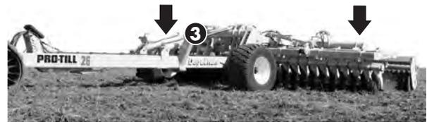
E. Place both the Transport Cylinders (#3) and the Wing Cylinders (#2) into the FLOAT position before operation.
