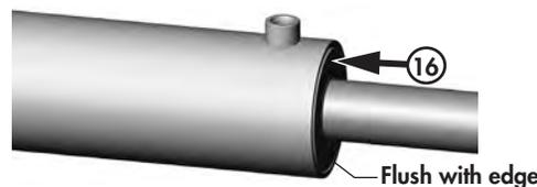
**IMPORTANT:** The head/gland must be inserted until it is flush with the tube to allow the inner wire ring to snap into its seated position in the internal cylinder groove. Failure to insert the head flush as shown will result in the head and rod assembly coming out of the tube when pressure is applied to the cylinder.
