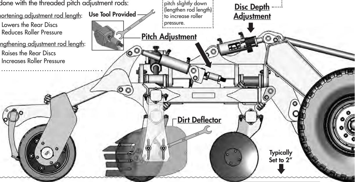
Adjust "Dirt Deflector Angle" whenever the Pitch of the Frame is adjusted.
