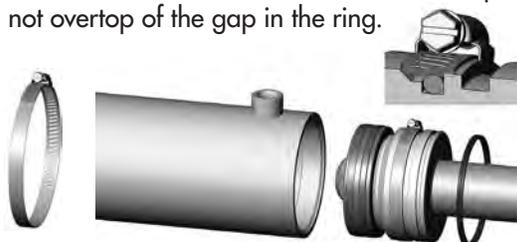
b) Tighten the band clamp to ensure the wire ring is fully seated. Then, loosen the clamp approx. 1/2 a turn to allow band clamp to slide during final assembly.
