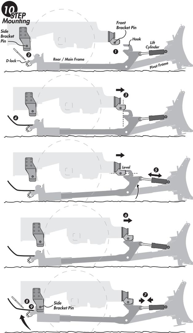
**⚠ Important:** There should be a gap (3/8" or larger) between the inside of the hook to the front of the bracket pin. The amount of gap may vary between specific models, but having a gap at this location is important.
