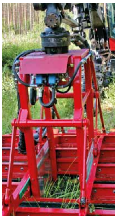
Naarva P55 uprooter presses unwanted saplings between rubbers with its jaws and roots them out of the ground.
