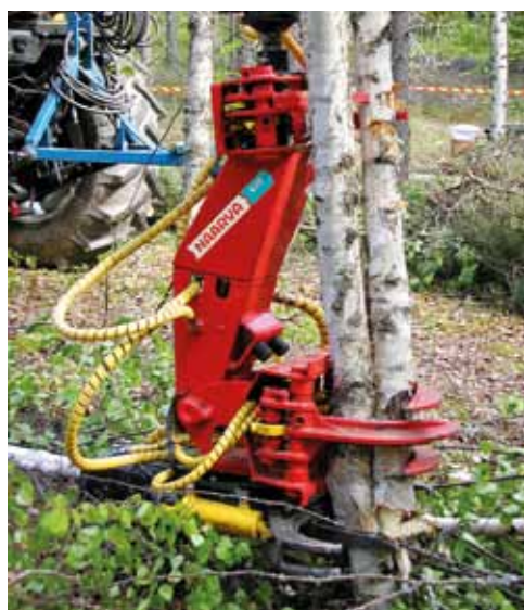
Naarva E20 with the strong Ø23 cm guillotine and higher accumulating grippers.
