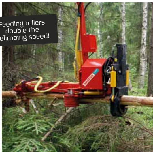
Stroke harvester with feeding rollers has four available delimbing speeds and forces.
