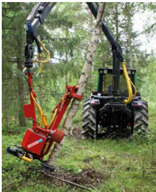
Naarva S25R has mechanical, cable-driven feeding rollers.
