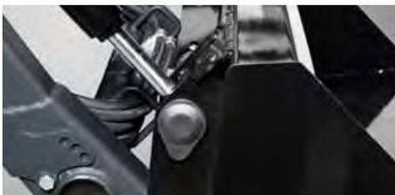
**3 | PIN-FIXING FOR IMPLEMENTS FOR 100C AND 140C.**
