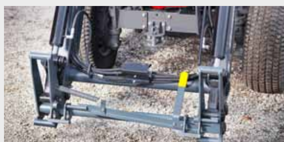
5 | CROSS TUBE IN UNIQUELY LOW POSITION.
