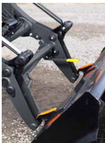
4 | QUICK ATTACH TOOL CARRIER FOR 160C AND 180C.
