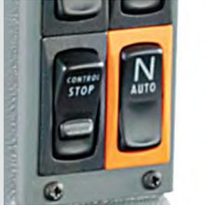
Valtra's excellent Autotraction feature is standard on A Series HiTech models. When Autotraction is activated, the tractor can be stopped from normal working speeds (below 12 km/h) simply by applying the brakes or lifting your foot from the gas pedal. The tractor then starts again when you release the brake or increase the revs. An electronic drive clutch developed by Valtra ensures smooth yet rapid starts.
