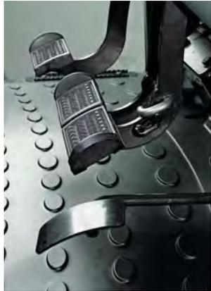
Entering the cab of A Series HiTech models is easy. The doors open wide, and the grab handles and steps are sturdy. Thanks to a highly adjustable steering wheel (reach and rake) and driver's seat, it is easy to find a comfortable driving position. Suspended pedals increase foot space, and the flat floor is easy to keep clean.
