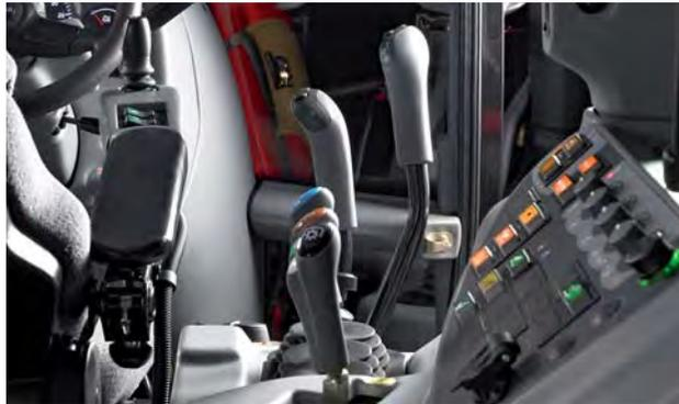
*The N Series lets you choose between mechanical or electronically controlled hydraulics. Controlling the hydraulics is straightforward and logical. The hydraulic oil change interval is 2000 hours, which saves time and costs. The N Series also allows for the optional use of bio-oils.*
