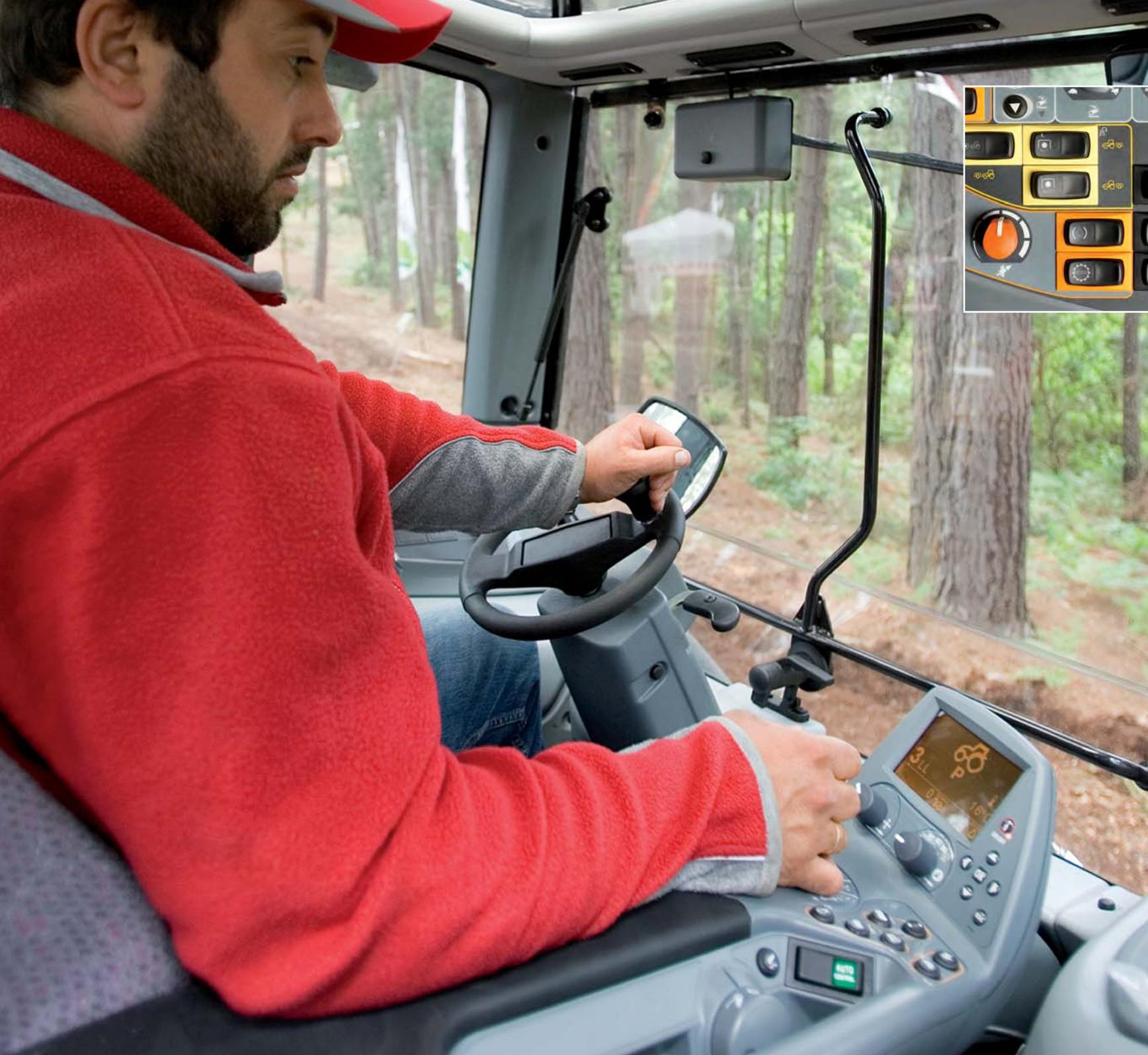
*The new design and positioning of the switches on the side panels combined with the use of colour coding makes them easy to use.*
