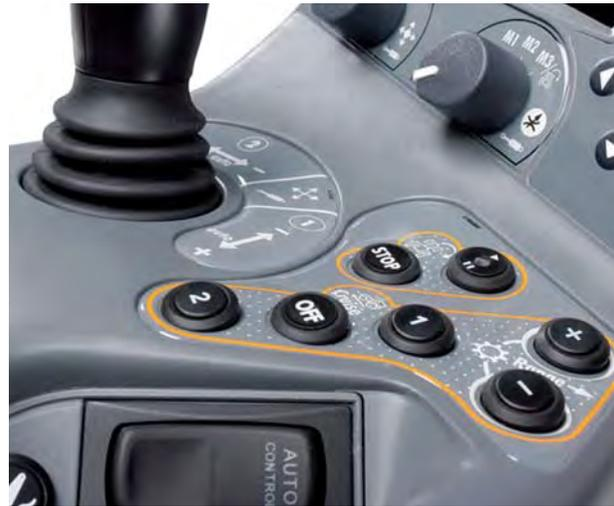
When working all you have to do is select the appropriate driving range and let the tractor take care of the optimal efficiency between the engine and transmission. If needed you can also set the engine speed or driving speed, either together or individually.
